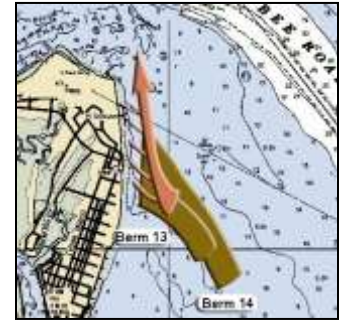
Strategic placement nearshore berm at Tybee Island, GA
