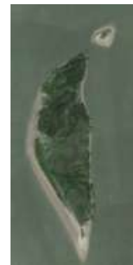
Island in the Atchafalaya River created by strategic upstream placement of dredged sediment
