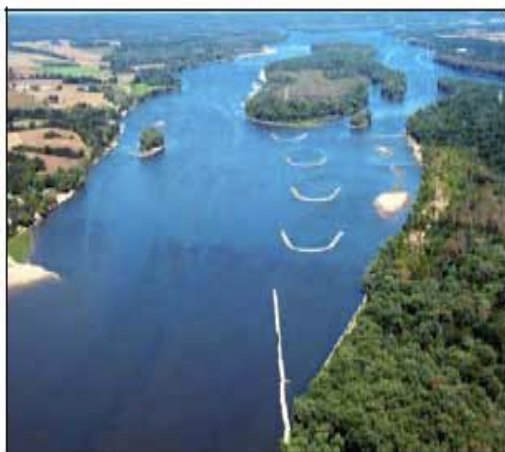
Figure 15. Aerial views of chevrons used in river engineering. (Photos courtesy of USACE Rock Island District)
