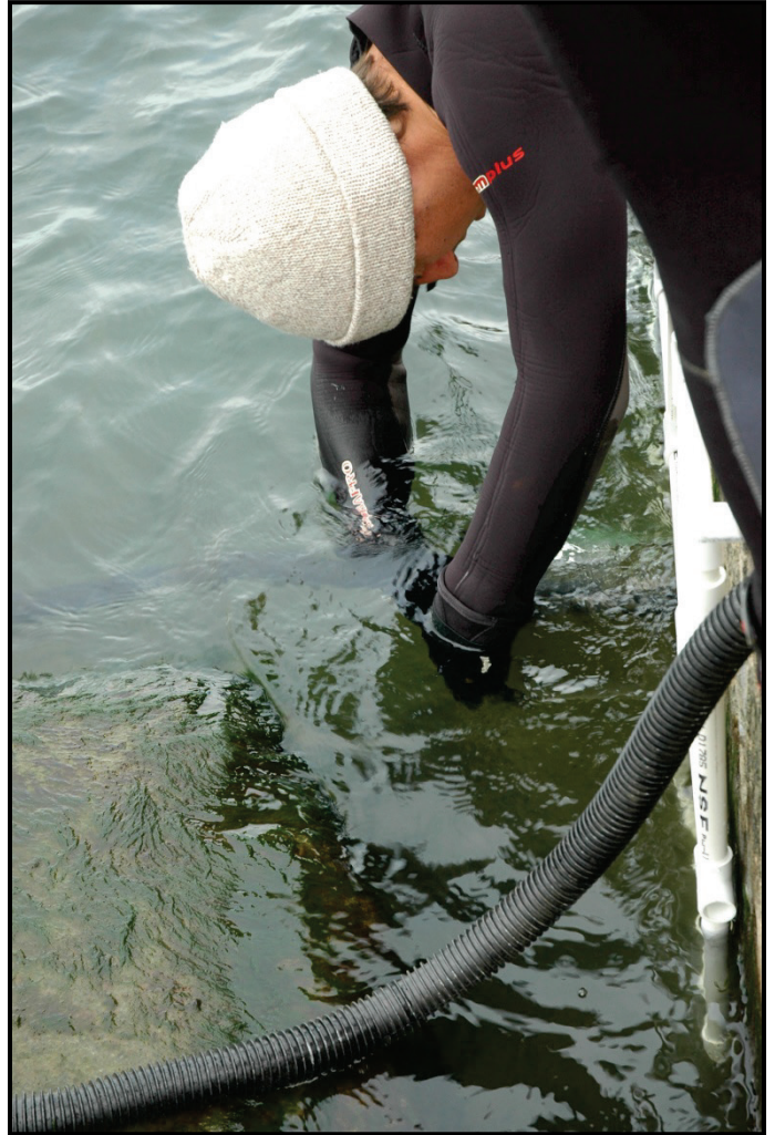
Figure 10. Sampling a toe block using the Plexiglas sampler, scraper, vacuum, and the PVC pipe sampling grid (photo T.J. Fredette).
