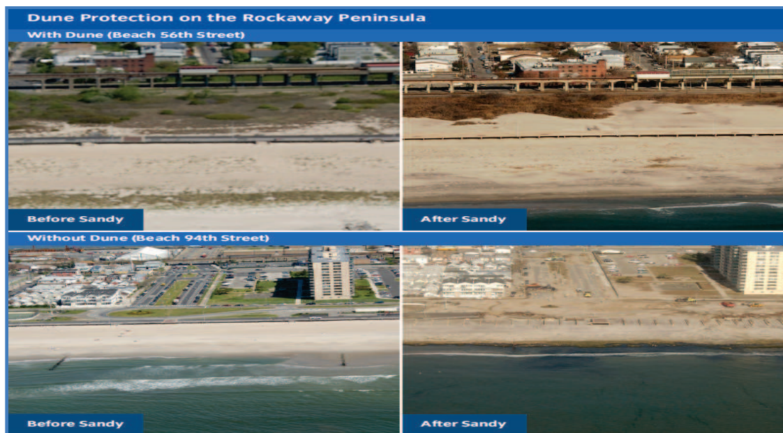
Figure 16. An example of NNBF performance was seen on the Rockaway Peninsula in Queens, NY (USA) after the storm. The pictures on the top compare a site with NNBF structures (i.e., dunes) offering a level of protection to the inland communities, whereas the picture on the bottom compares a site absent NNBF (Source: http://www.nyc.gov/html/sirr/html/report/report.shtml ).
