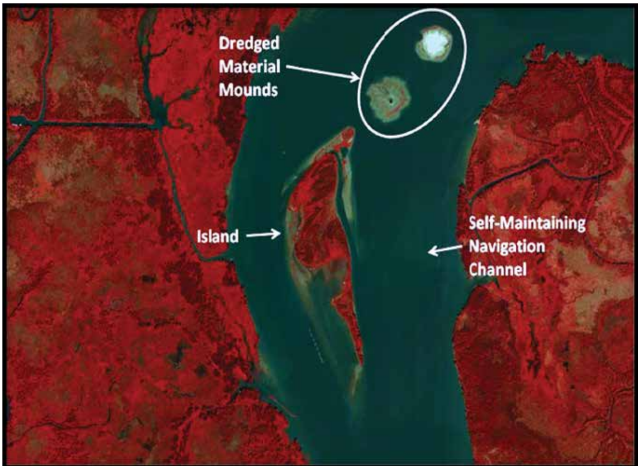
Figure 1: December 2011 aerial infrared photograph of the Atchafalaya River island after multiple years of upstream mounding of dredged material. The island's formation has reduced the overall cross sectional area of the river, increasing river flow through the navigation channel to the east sufficient to reduce shoaling and maintenance dredging requirements.
