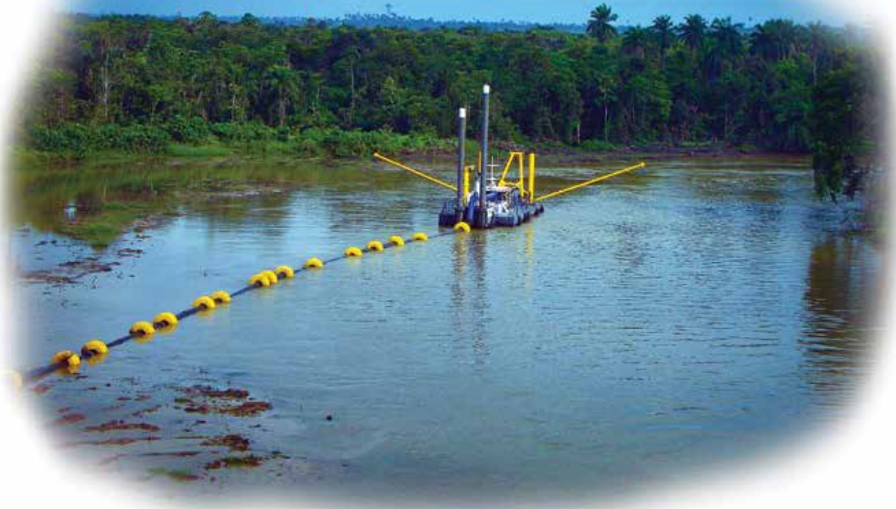
CSD500 Karamara on site eating away through the sand banks blocking the river
