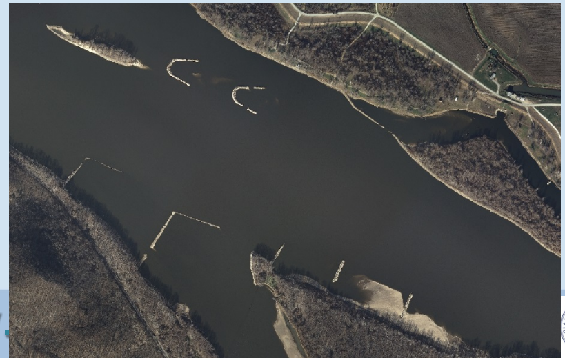
Aerial view of chevrons at Bolters Bar. Note sand bar islands created downstream from the chevron structures.
