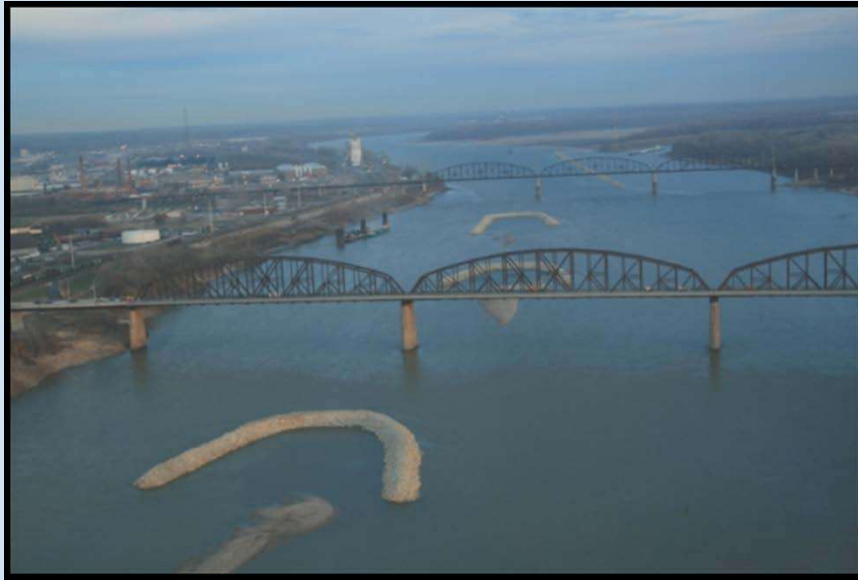
Aerial view (looking upstream) of three chevrons at St. Louis Harbor. Note sand bar island, a habitat used by many wildlife species, created downstream from the middle and nearest chevron structures.
