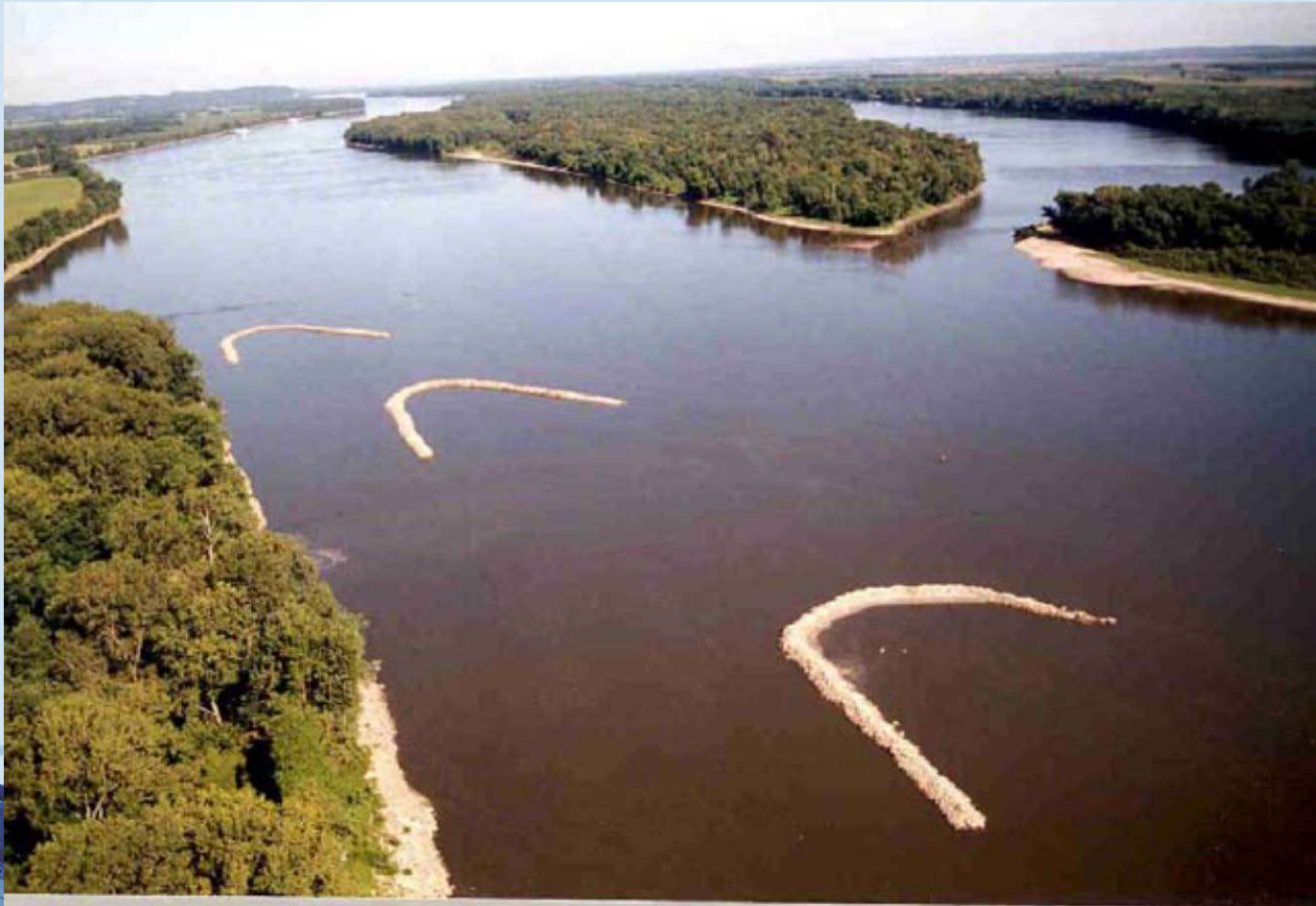
Blunt Nosed Chevrons at Miss. River Mile 266 USACE St. Louis District, Applied River Engineering Center
