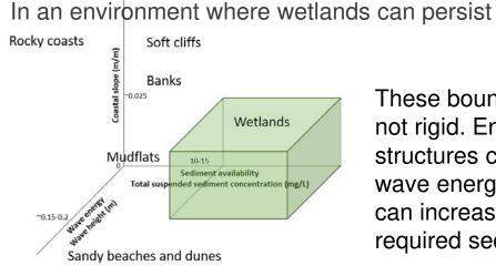
These boundaries are not rigid. Engineered structures can modify wave energy and SLR can increase the required sediment.
