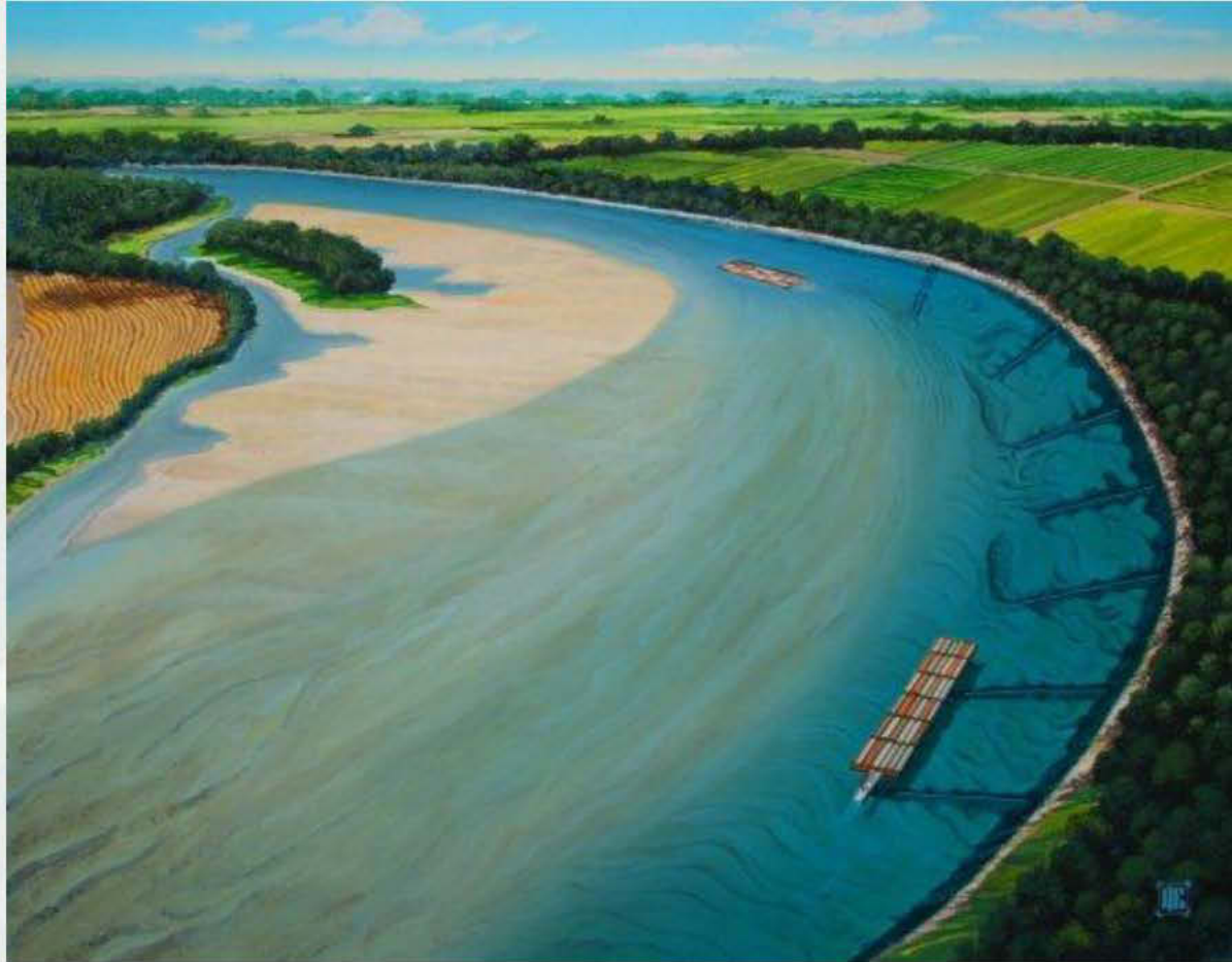
River Bendway Weirs
