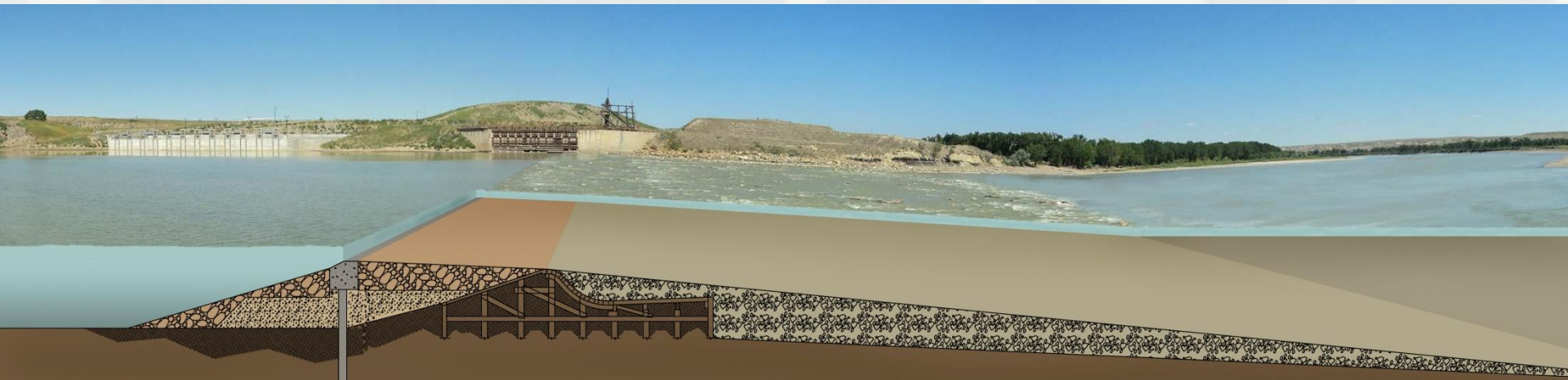
LOWER YELLOWSTONE INTAKE DEEP FOUNDATION WEIR
