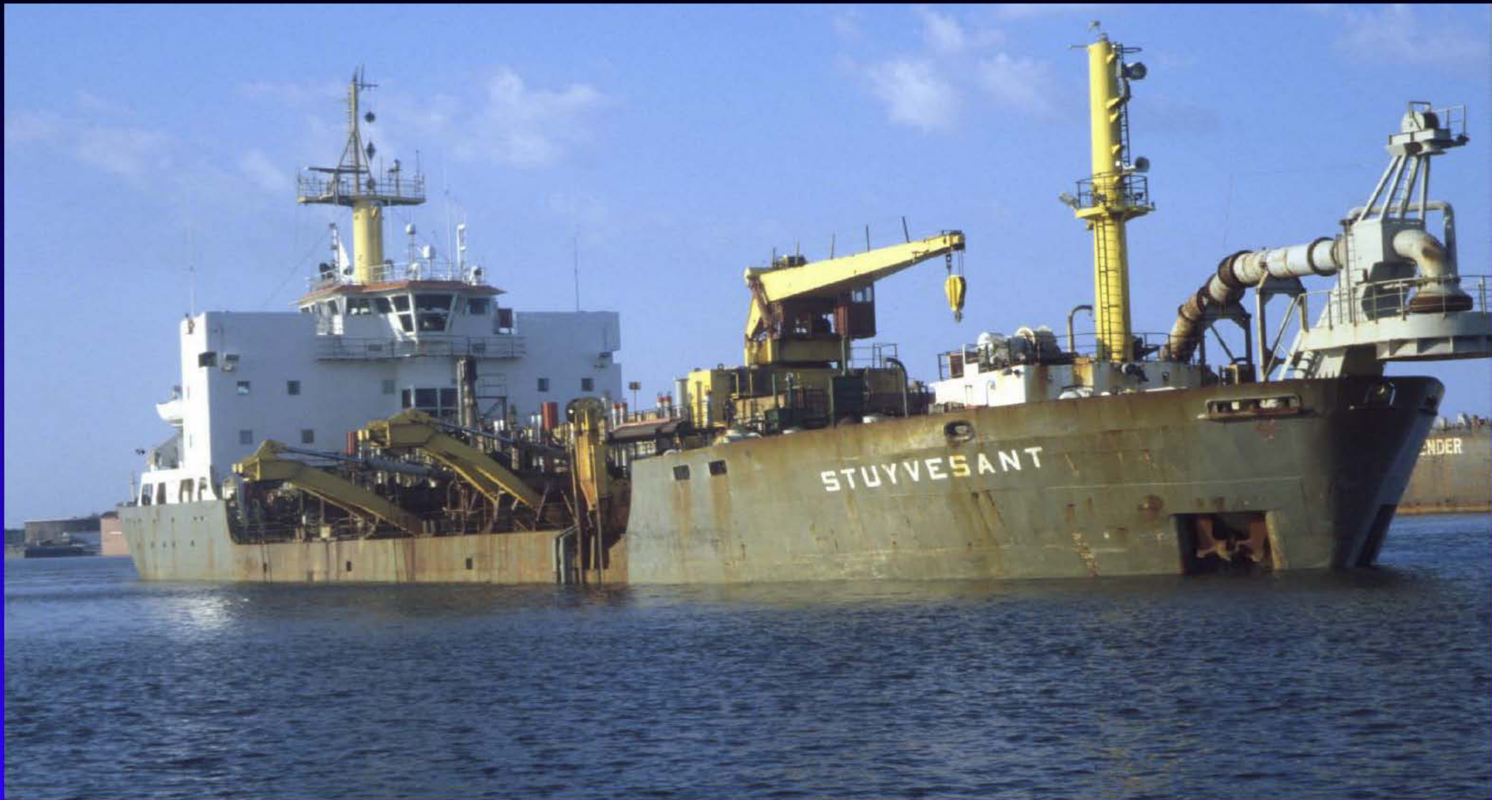
Bean Stuyvesant Hopper Dredge Stuyvesant (15,000hp, 11,140 cyd) Operating in Mobile Bay, Alabama
