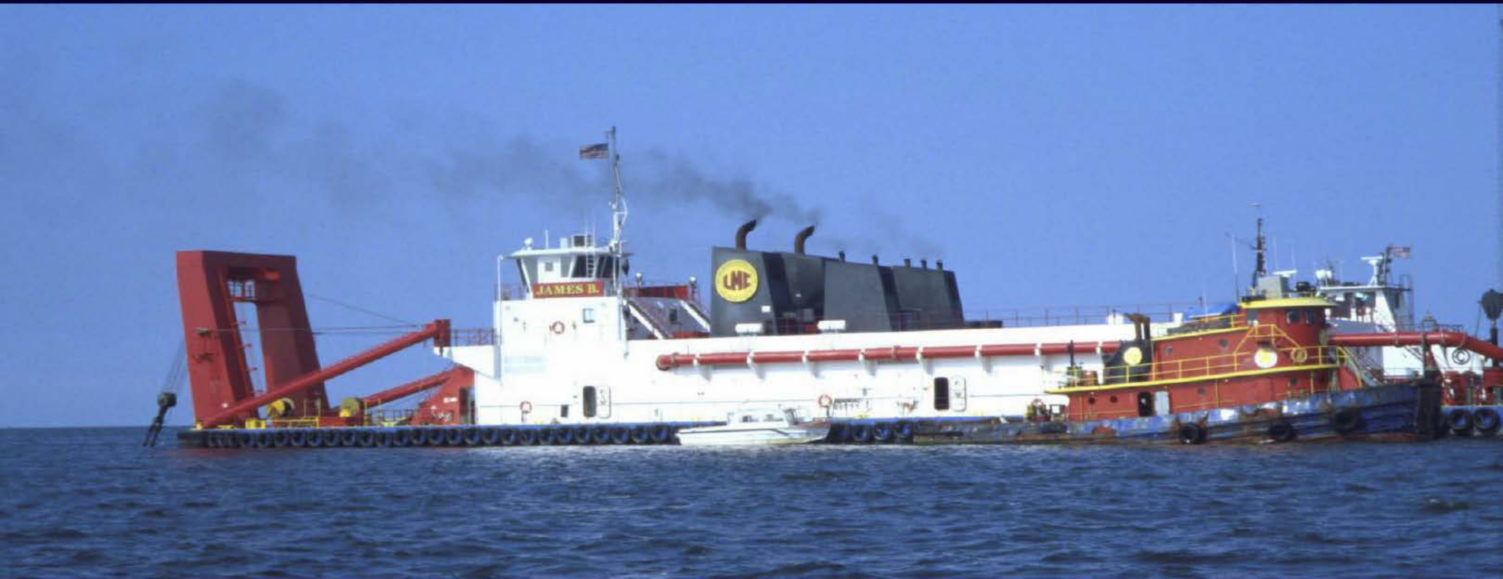
LMC Hydraulic Cutterhead Dredge James B (24", 10,000hp) Operating in Mississippi Sound off Gulfport, MS
