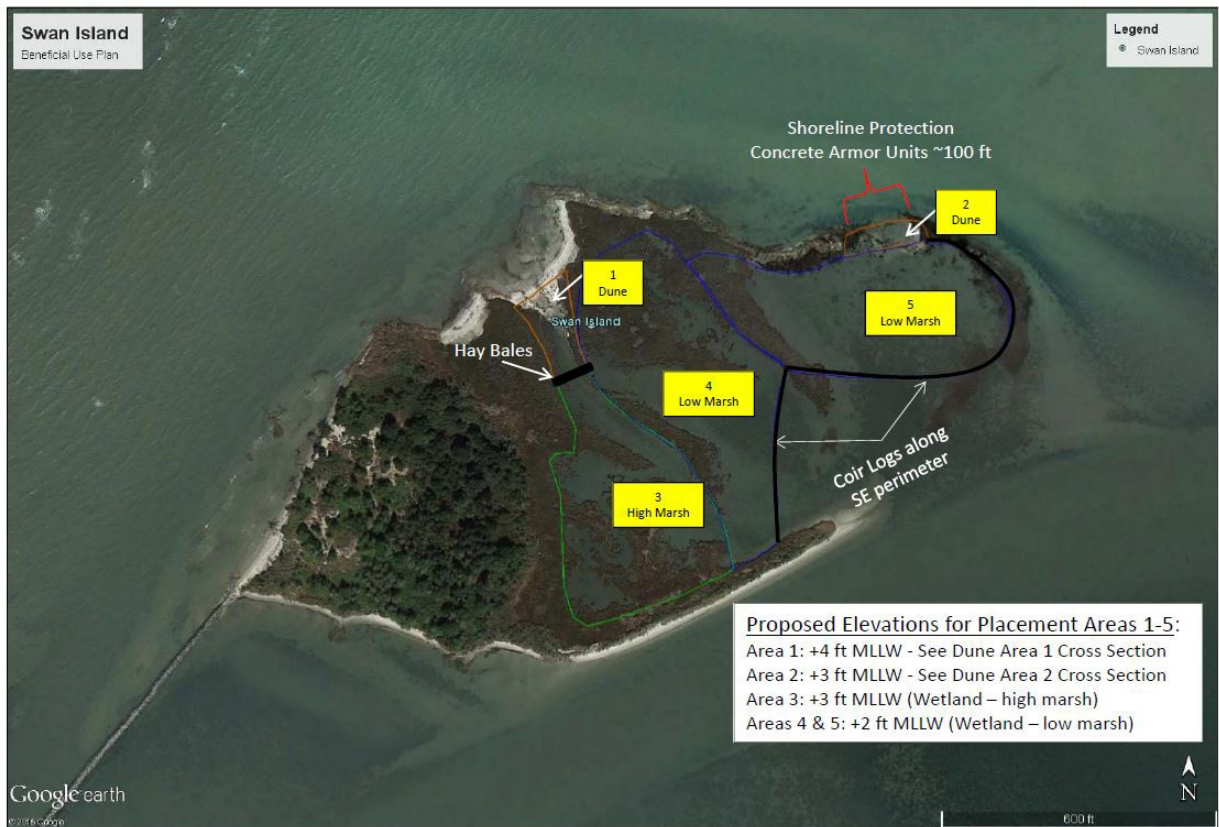
Figure 2. Google Earth image of Swan Island, with the beneficial use plan overlaid. Natural and nature-based features to be restored include low marsh, high marsh, dunes and strategic use of concrete armor units (image from: Environmental Assessment Twitch Cove and Thorofare Federal Navigation Channel Project, Dec 2015)
