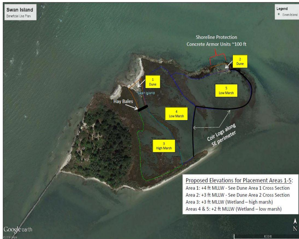
Figure 6. Google Earth image of Swan Island, with the beneficial use plan overlaid. Natural and nature-based features to be restored include low marsh, high marsh, dunes and strategic use of concrete armor units (image from: Environmental Assessment Twitch Cove and Thorofare Federal Navigation Channel Project, Dec 2015)
