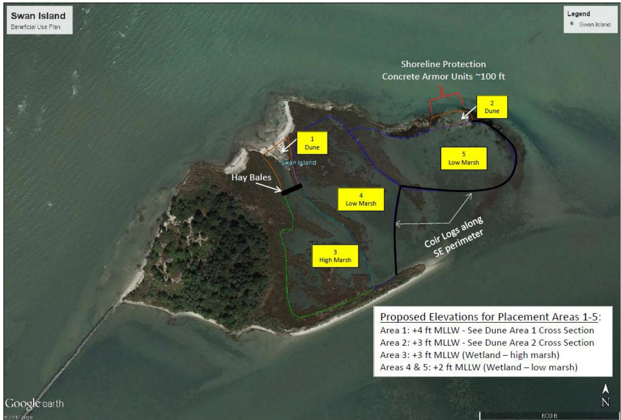
Figure 2. Google Earth image of Swan Island, with the beneficial use plan overlaid. Natural and nature- based features to be restored include low marsh, high marsh, dunes and strategic use of concrete armor units (image from: Environmental Assessment Twitch Cove)
