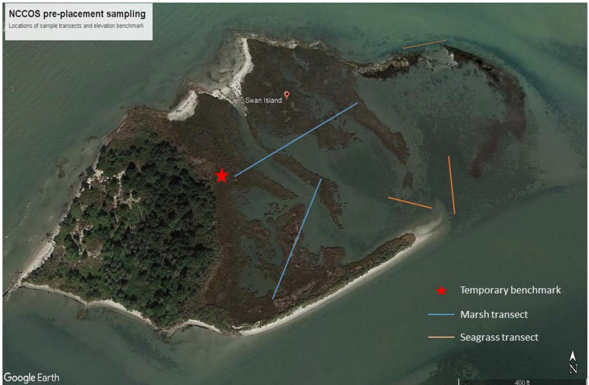
Figure 3. Satellite image of Swan Island indicating the location of the temporary benchmark and the marsh and seagrass transects surveyed in August 2018, prior to restoration of the islands natural features with the placement of dredged sediments.
