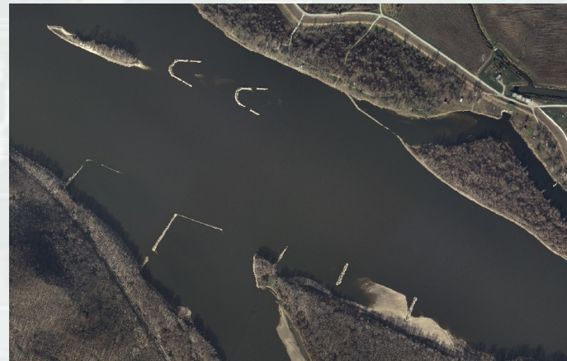
Aerial view of chevrons at Gilbert. Note sand bar islands created downstream from the chevron structures.
