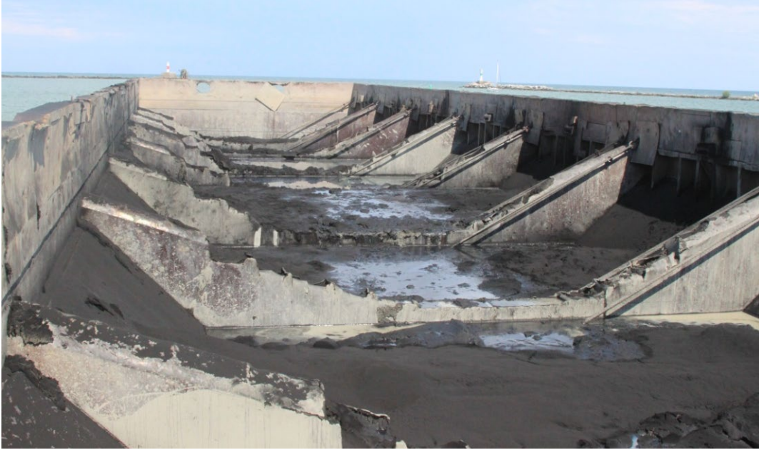
Figure 1. Dump scow for open water placement of dredged material.
