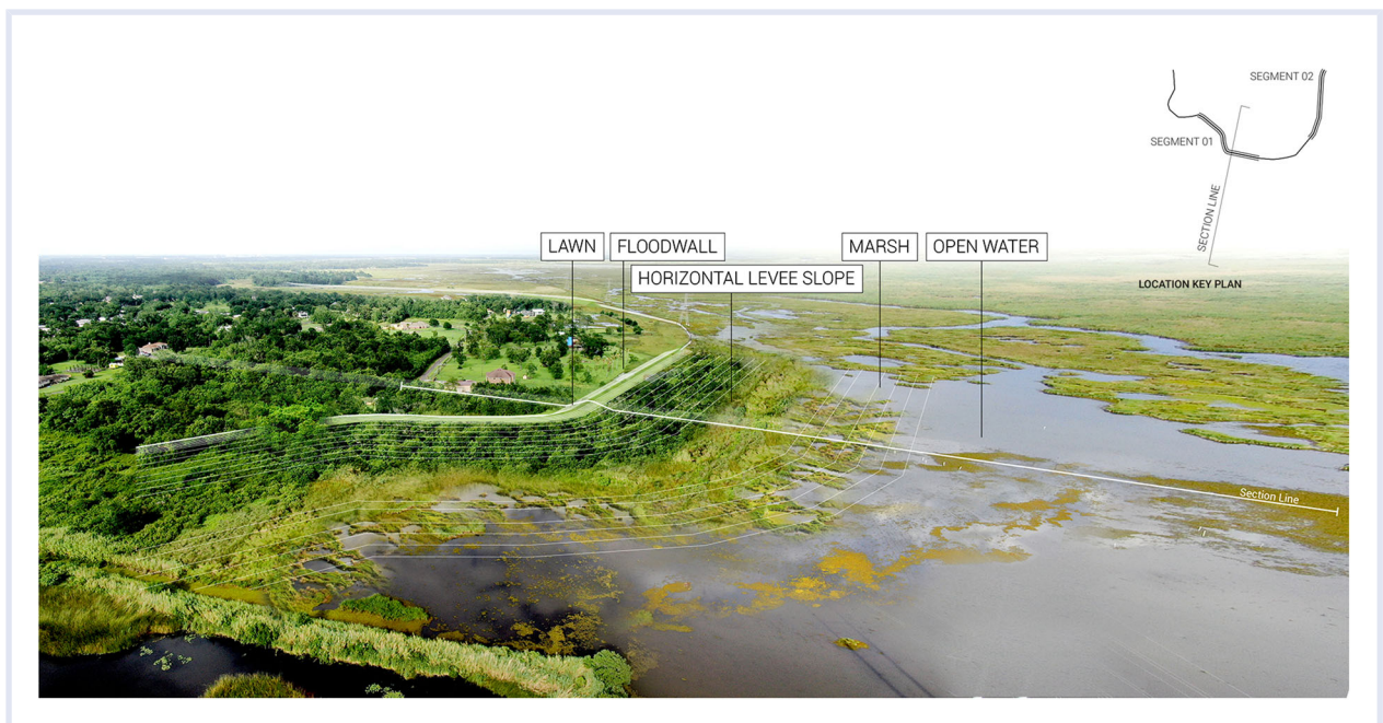
FIGURE 4 Aerial perspective view of potential horizontal levee implementation in Bridge City (Orange County), Texas
