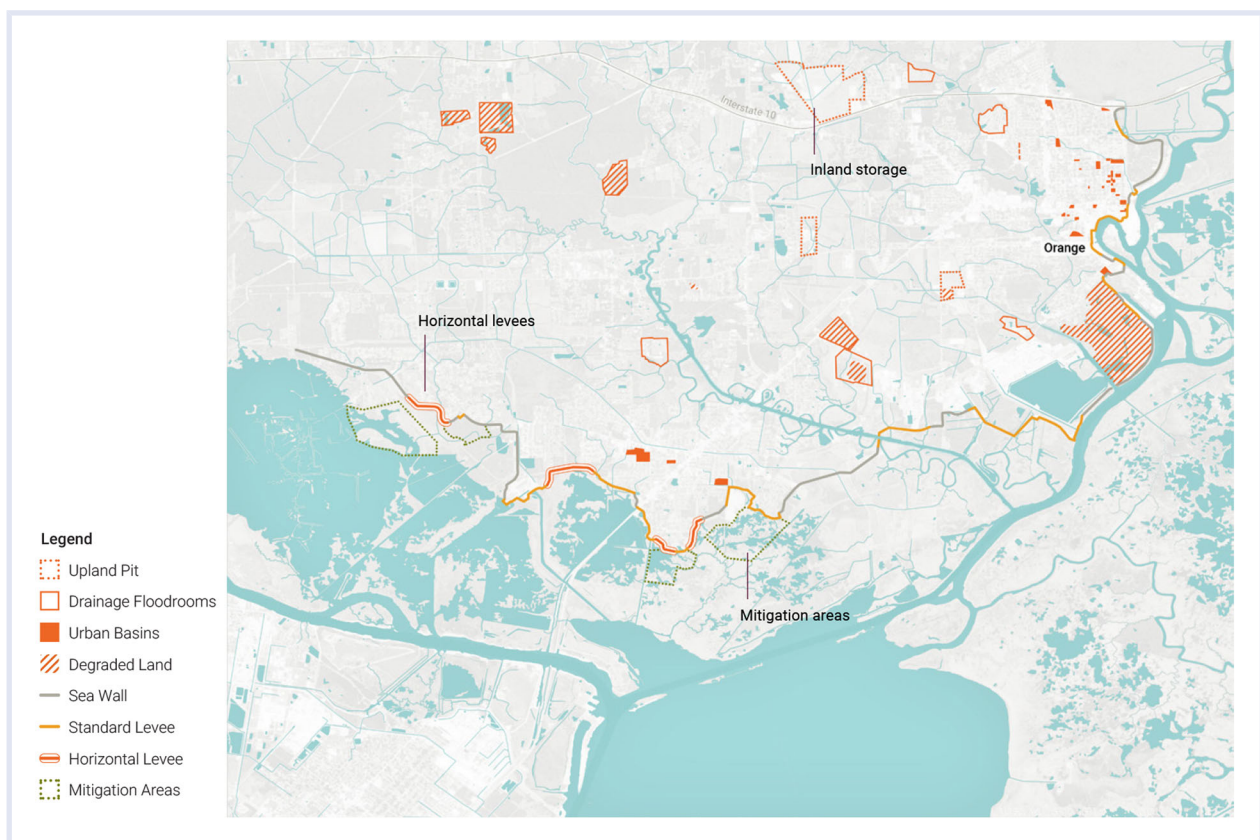
FIGURE 2 Potential locations of natural and nature-based features in relation to the proposed Orange, Texas, Hurricane Flood Protection System
