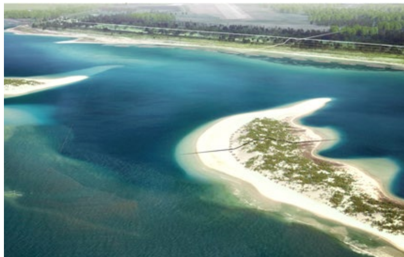
Above: For protecting inland assets from coastal flooding, nature-based solutions include enhanced sand trapping on the barrier islands and dune construction along the mainland. (Photo by Jacobs)
