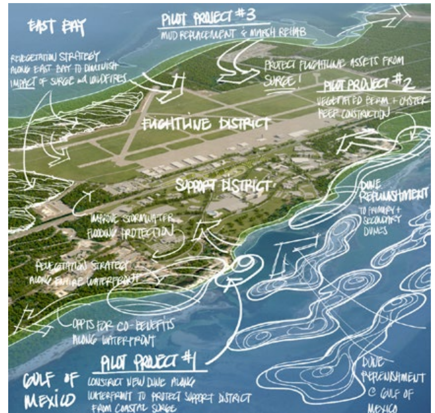
Above: Drawing of various EWN approaches superimposed on an aerial image of Tyndall AFB. (Image by Brett Wylie, Jacobs)
