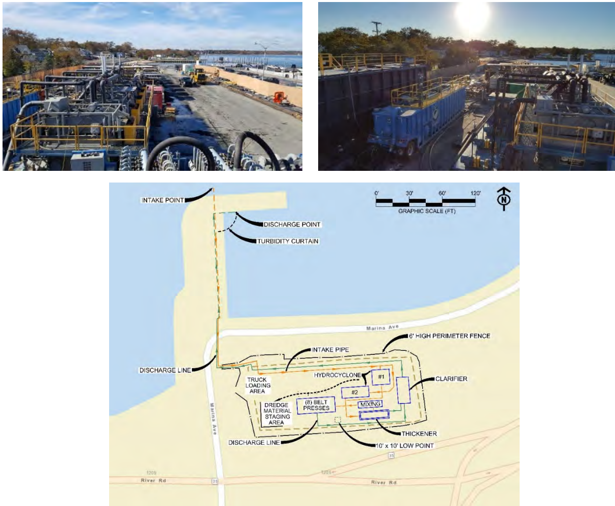
Figure 5. Photograph and equipment layout for active dewatering system used in Phase II.
