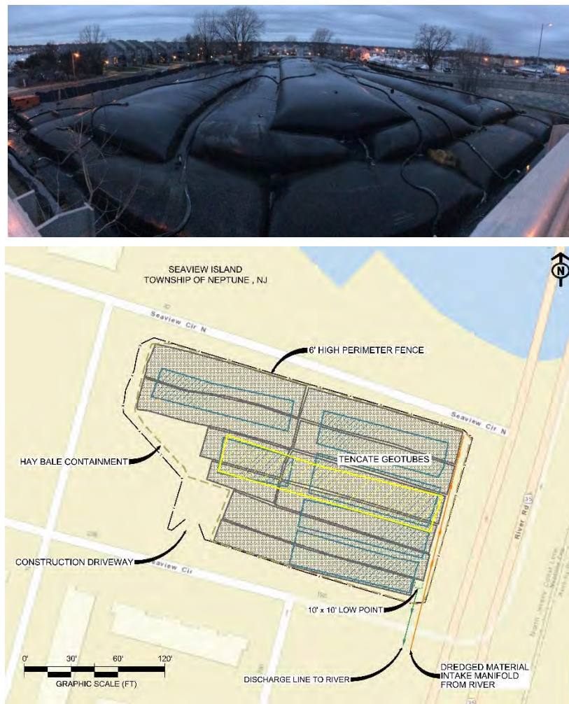
Figure 4. Site layout and photograph of Phase III passive dewatering system
