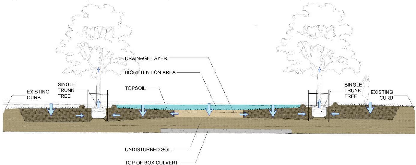
Figure 5. Cross-sectional rendering of the primary components of the bioretention areas of the project. Arrows mark surface and near-surface water flow designed to reduce flood risk.
