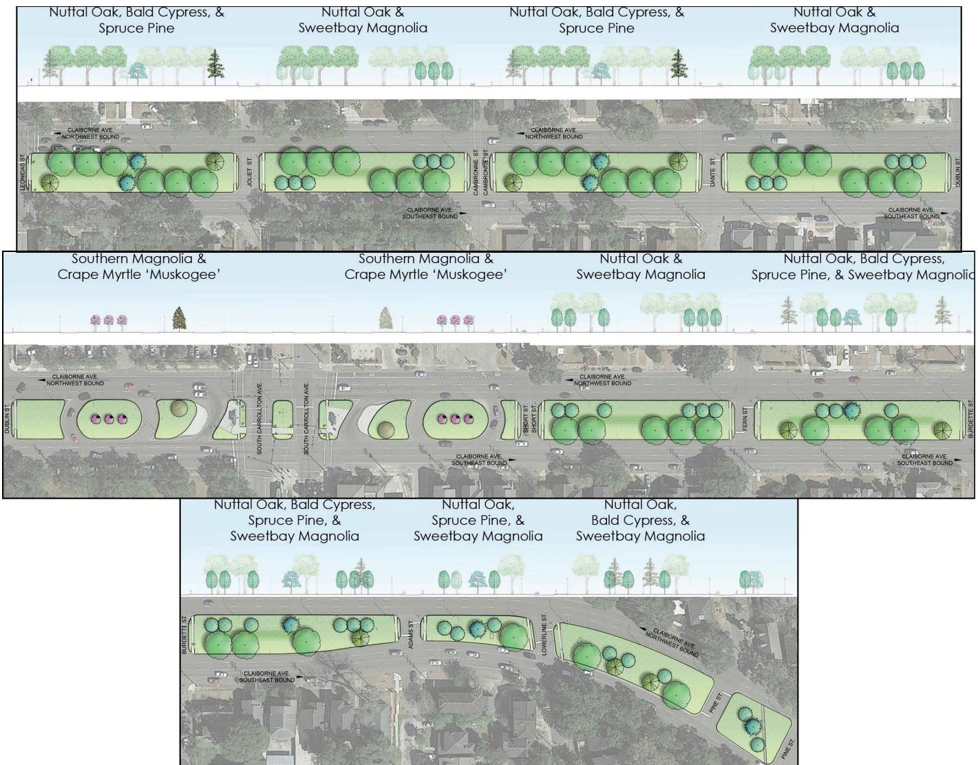
Figure 6. The scaled plan and elevation renderings for the greenspace restoration of South Claiborne Avenue demonstrate the planting design and rhythm of the native street trees that a driver may experience passing at 56 kmh (35 mph).
