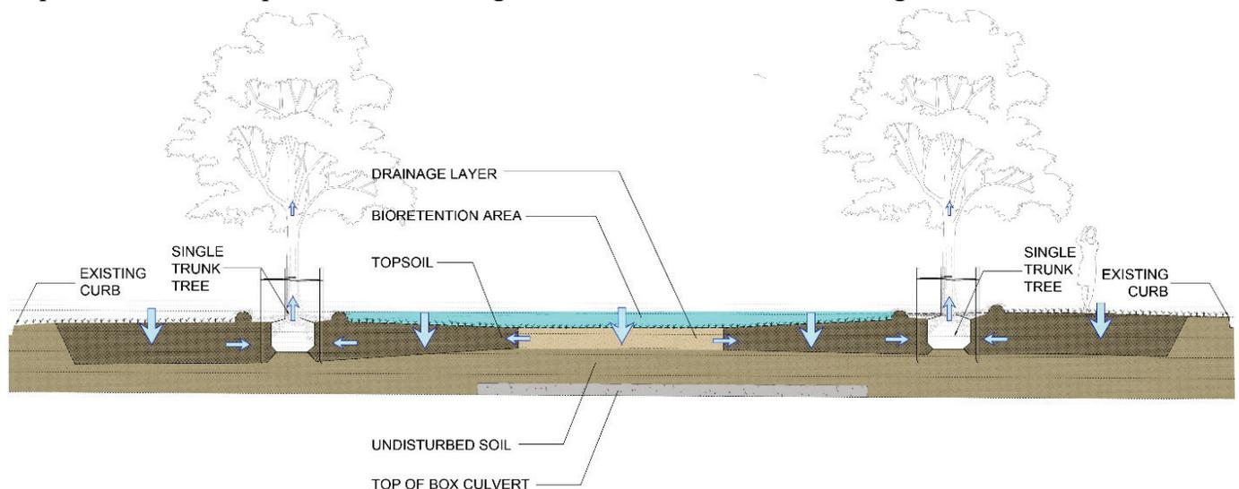
Figure 5. Cross-sectional rendering of the primary components of the bioretention areas of the project. *Arrows* mark surface and near-surface water flow designed to reduce flood risk.
