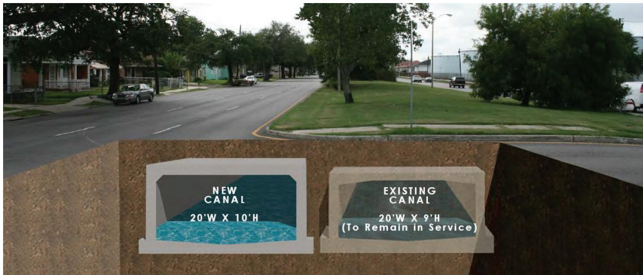
Figure 2. On South Claiborne Avenue, a new canal was constructed next to the existing underground canal (culvert) below the neutral ground.
