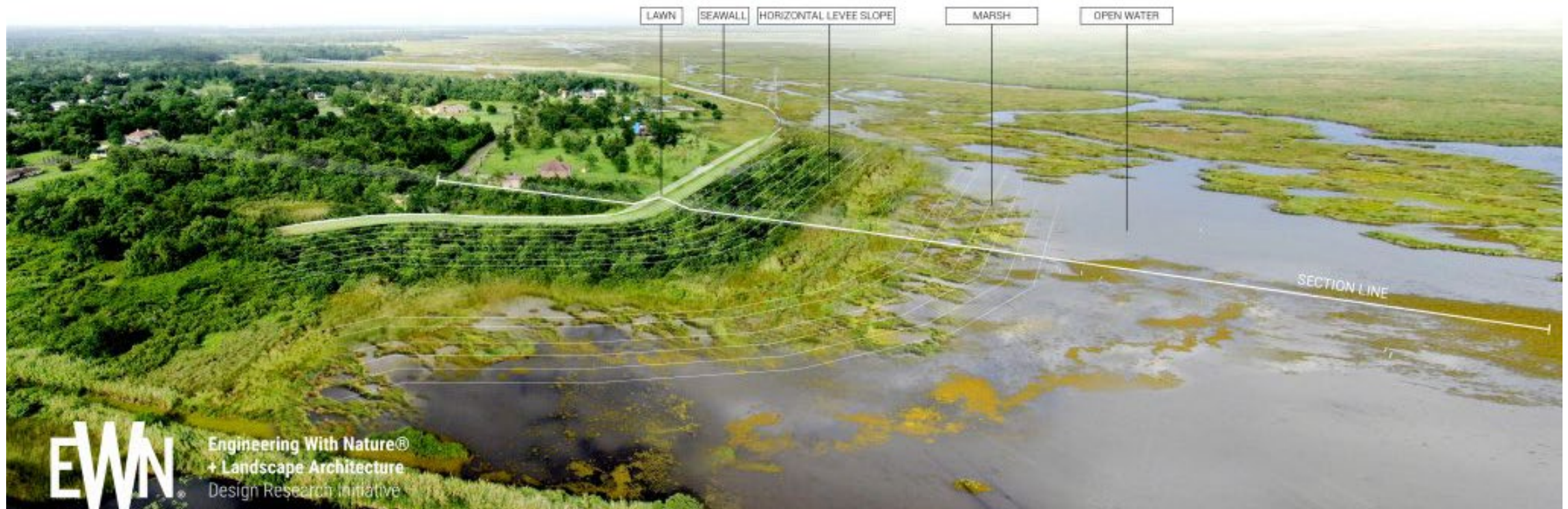
A rendering of a horizontal levee design that achieves storm and flood risk reduction while increasing habitat value.
