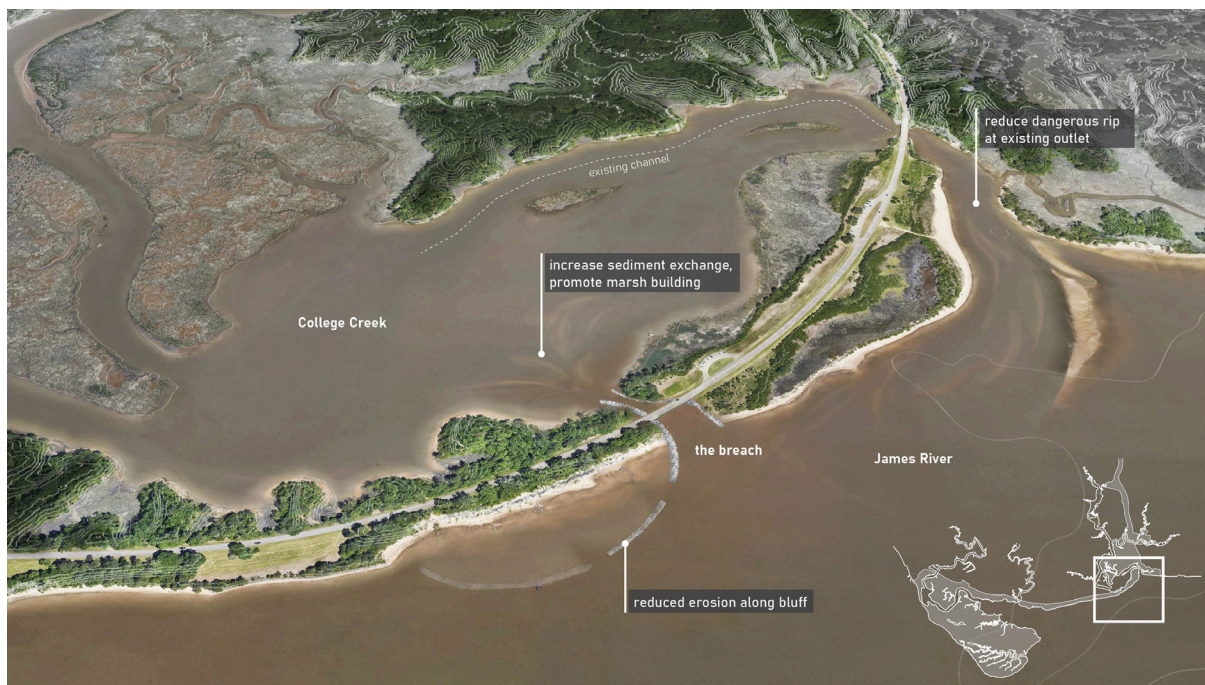
Figure 3. The Breach, aerial perspective rendering. Illustrates how proposal would facilitate exchange of water and sediment between James River and College Creek.
