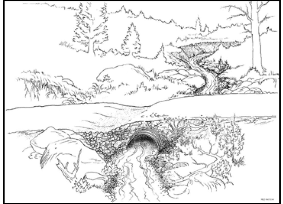
Figure 3.2 Conceptual rendering of a cylindrical culvert with an over topping roadway spillway that can integrate scour protection.
