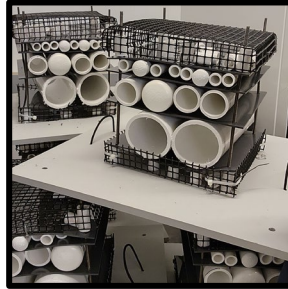
Fish-specific Autonomous Reef Monitoring Structures (FARMS)
